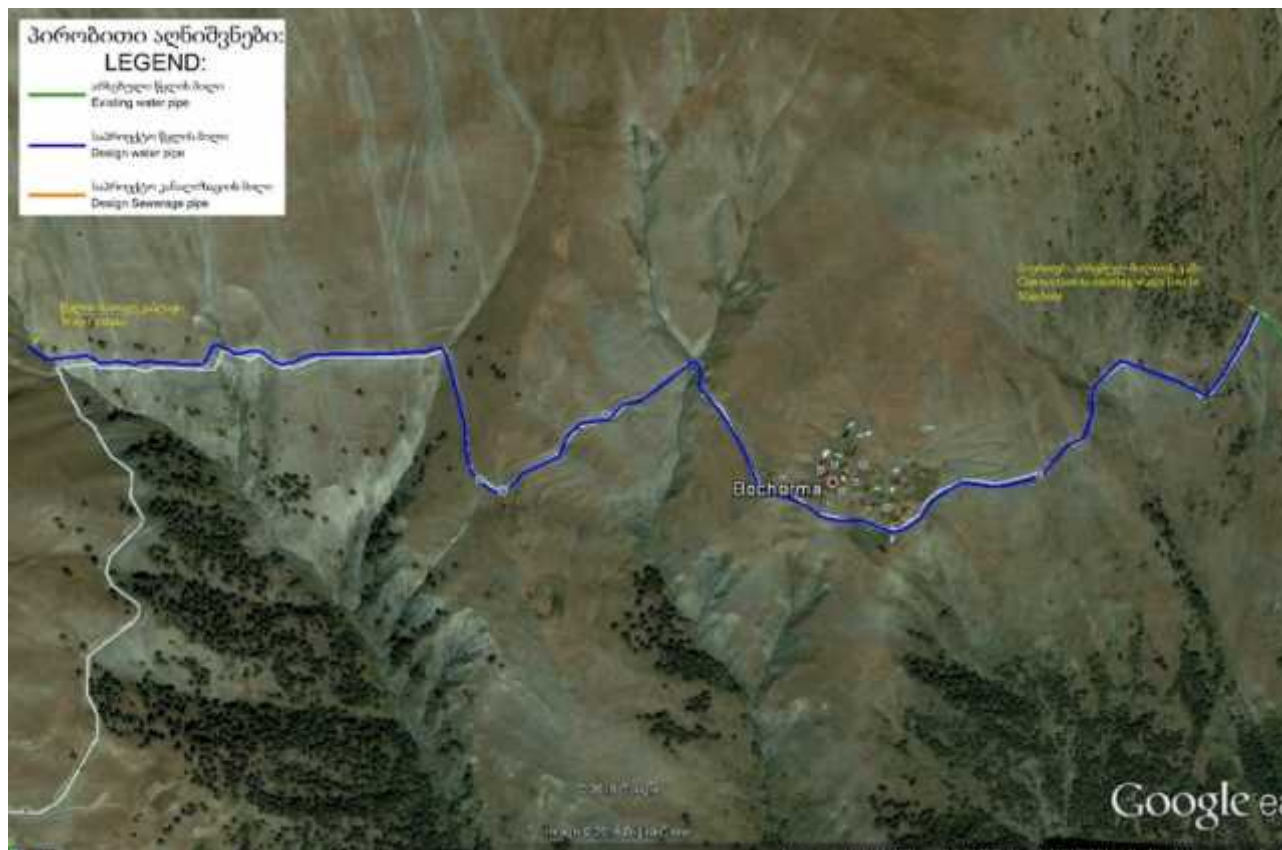
Map 2: Arrangement of additional water source and a supply system from that source to the existing water collector chamber
