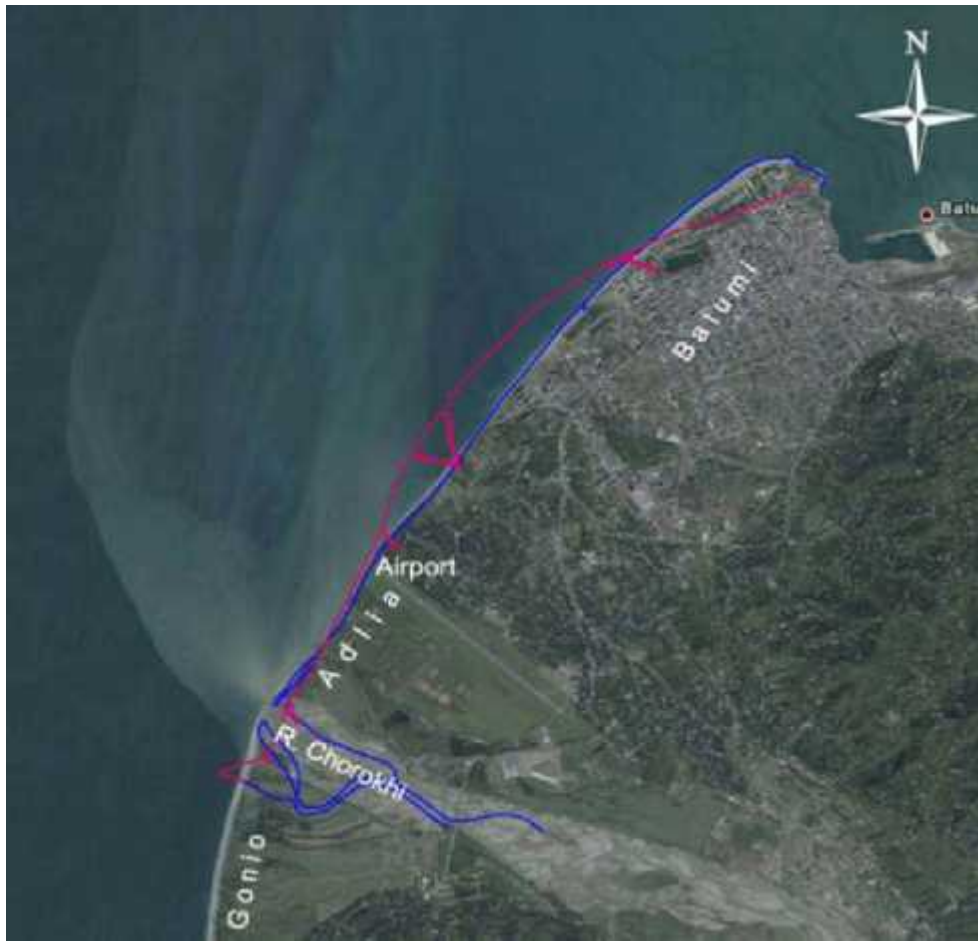
Fig. E.9: Coastline (blue) of Batumi and the coastline of 1830 superimposed in red.
