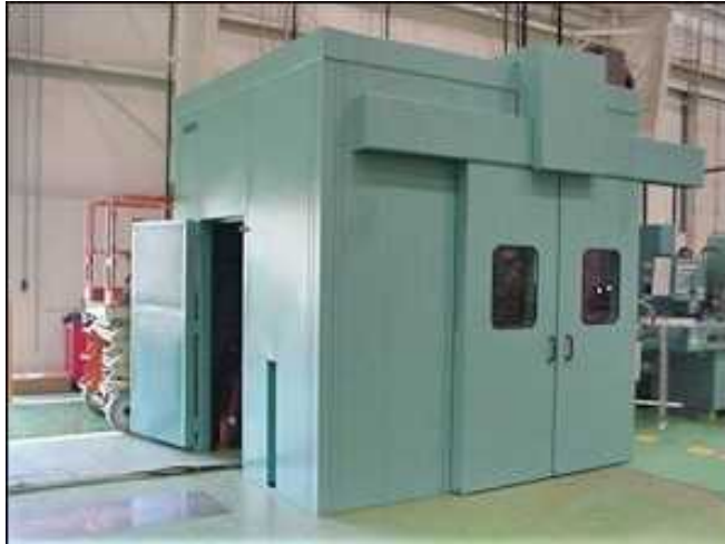
Fig. F.5: example of soundproof enclosure
