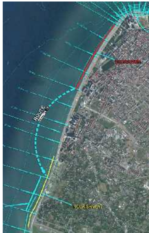
Fig. G.3: Schematization of the excavation – nourishment process
