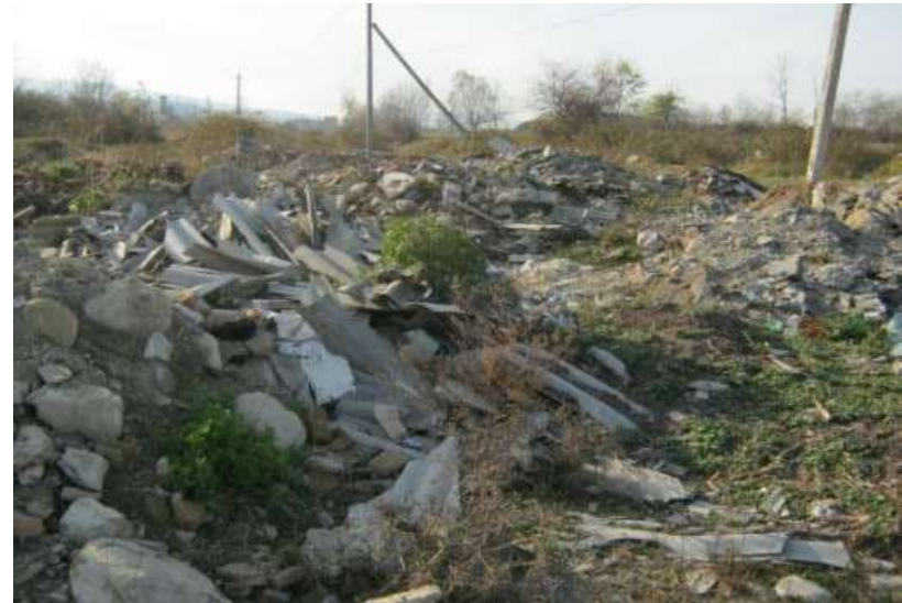
Site 2 – Fragments of asbestos-cement tiles.
