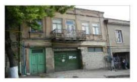
House # 39 (Cultural Heritage Monument<sup>6</sup>) The SP considers removal of existing plastering, re-plastering and painting. Replacement of roof rainwater drainage pipes on the roof; Restoration of doors and windows on the second floor and the main entrance door on the first floor. Replacment of large door and window on the first floor, finishing of the stair with basalt tiles at the main entrance of the building, cleaning and painting of the balcony railing.
