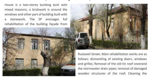
façade from old plastering using sand-jet blower, demolition of damaged elements, restoration of wall damaged fragments, installation of doors and windows, façade plastering with sand-cement mortar, installation the woodwn structures of the roof and roof cover with gray tin sheets, installation water collecting pipes, painting the doors and windows, arrangement of stair steps with basalt slabs.
