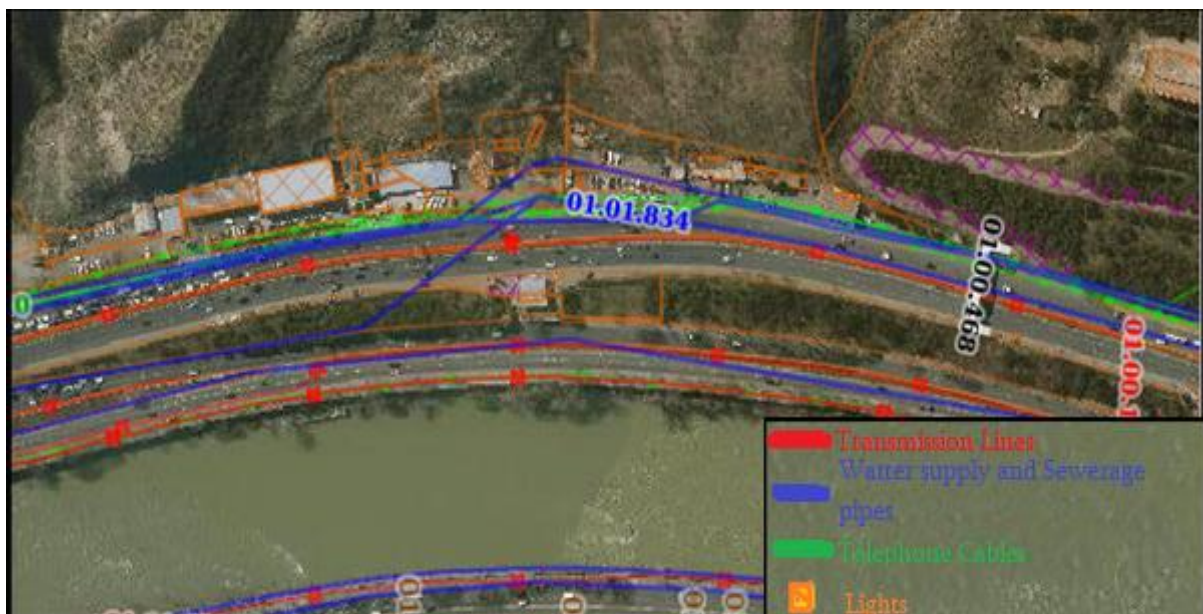
Figure 5: Locations of the water-supply and sewerage pipes, power transmission lines and lights in the project zone
