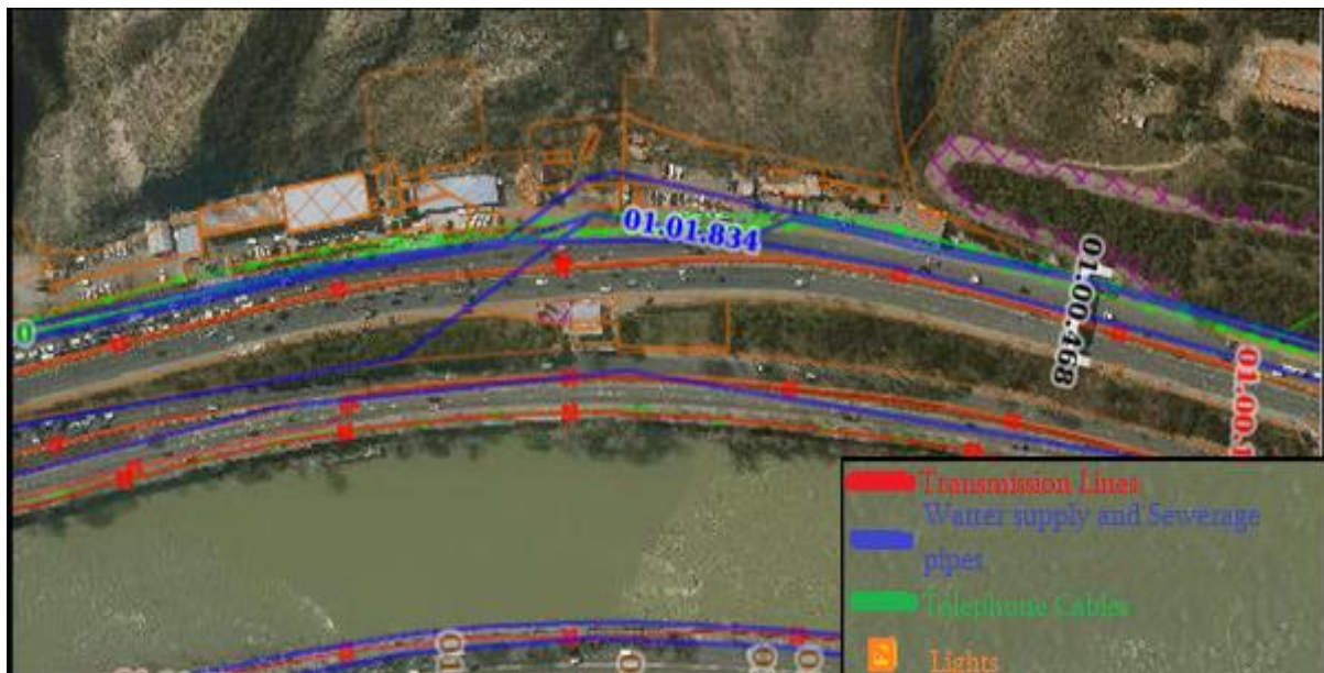
Figure 5: Locations of the water-supply and sewerage pipes, power transmission lines and lights in the project zone
