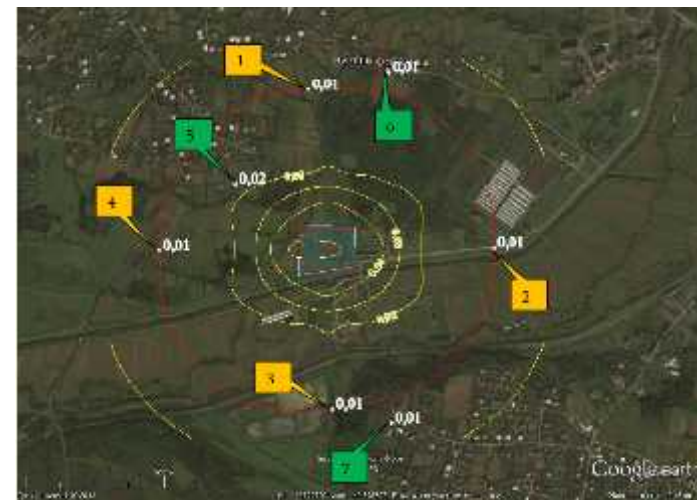
Maximum concentrations of total impact of the 6003 group (codes 303 +333) on the border of 500 meters zone (points № 1-4) and on the border of the nearest residential zone (points.№5-7).
