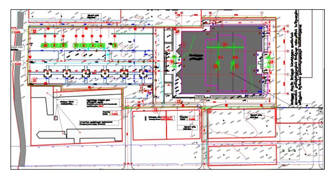
Figure 5. Construction site organization scheme: 1.Sport Complex; 2. Technical spaces; 4. Manager's room; 5. Dressing room; 6. Dining room; 9. Warehouse, 11. Temporary fence; 14. Open warehouse.
